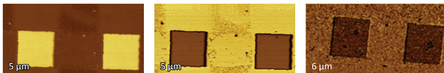
Height (left), IR reflection (center) images and dC/dZ map (right) of Si/SiO 2 grating
